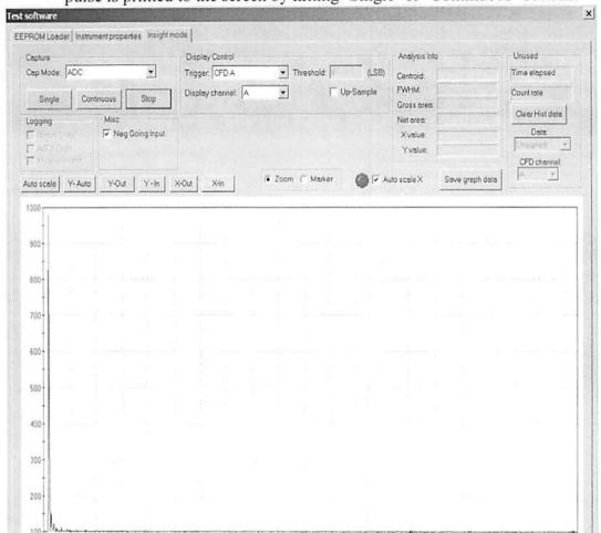
(vii)To visualize a train of pulses, choose "Snippet Data" in 'Cap Mode.' To record the data, **choose "Fast Capture"** instead, and hit 'Continuous' button. The pulses have to be recorded in ASCII format ('Logging' option "ASCII Data"). Approximately 300 MB measurement file will be acquired and stored at C:\.
