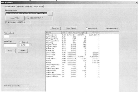
(v) Click on the text "PreTriggerTime" in the large white-background window. Rewrite the current value to "8" by using the small read/write window on the left-hand side. Before clicking on 'Write' button, make sure to mark the 'Decimal' option. In the same way, change the "PostTriggerTime" and "TrigThreshAU" values to decimal 8 and 110 (~100 keVee), respectively.
