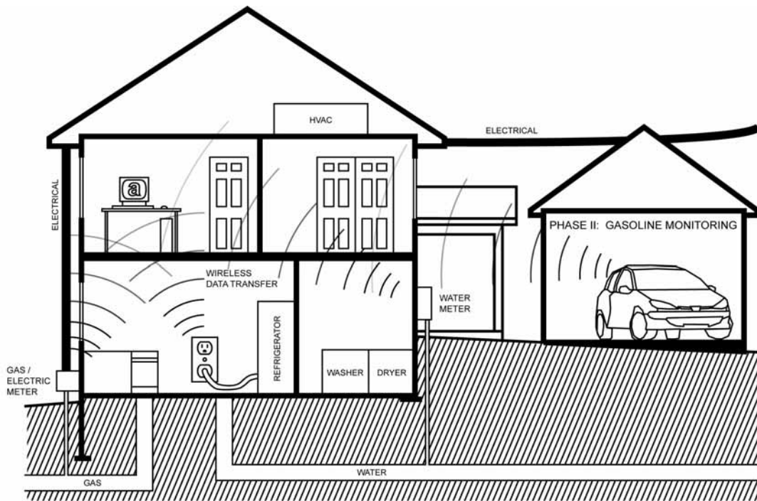
Figure B-4. Conceptual illustration of the AWARE@home system. Electronic accumulators and wireless transmitters connect to existing metering technologies (gas, electric, water). A USB-compatible receiver is utilized, along with a device to monitor & transmit electricity consumption of single appliances “plugged in to the wall”.
